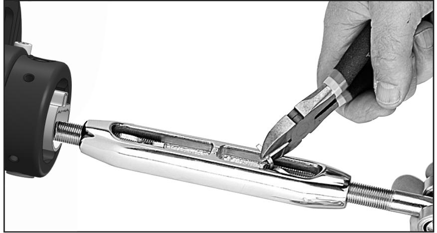
Slide lower drum assembly over turnbuckle and attach using long crosspin.
