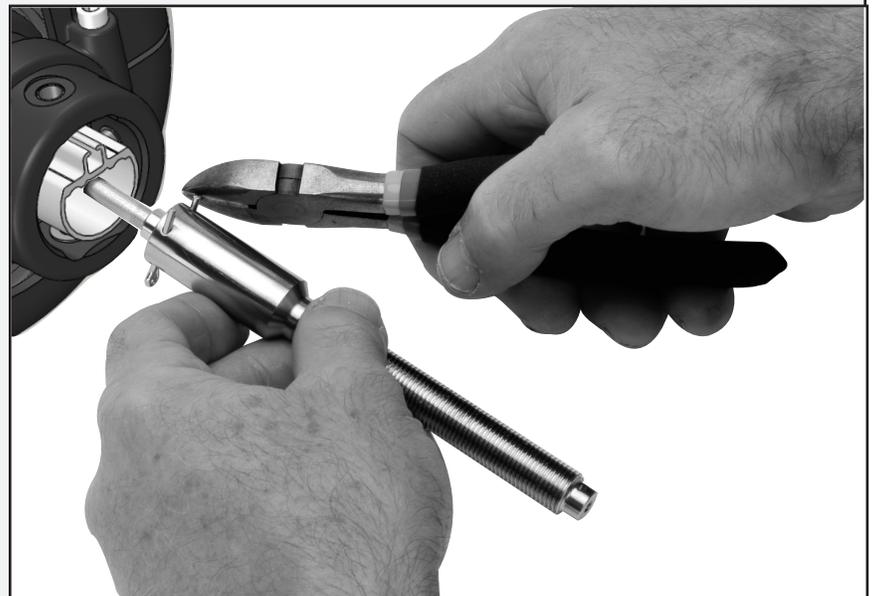
Assemble turnbuckle and attach Harken toggle.
